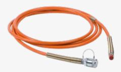
When working with high pressure hydraulics 700 Bar / 10.000 psi safety comes first. All Holmatro hoses are suitable for 700Bar working pressure. Our hoses are designed on a 4:1 safety ratio, resulting in a 10 year lifespan. All hoses are individually tested during the production proces.
