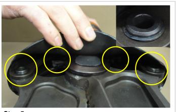
**Step 5**Check the 4 smalley rings for presence and damage.
