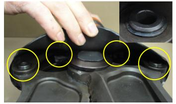
**Step 6** Check the smalley rings 4x for presence and damage.
